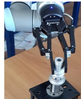
Figure 4. UR10 manipulator robot with 2F-140 adaptive gripper
